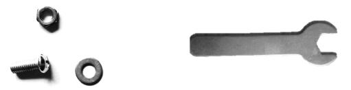
Install the panel from the front of the Volair Sim Chassis and align it to match the row of holes pre-drilled along the bottom edge of panel to the table. Use the provided four sets of screws and nuts to secure the avionics panel to the avionics table. Use the universal wrench to prevent the nuts from turning while tightening.
